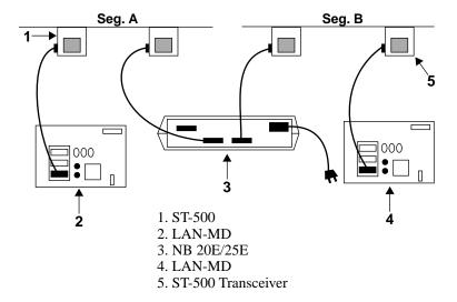
Figure 4-2 Check Out Configuration
